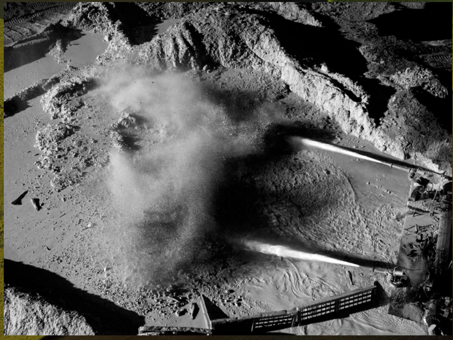
Clockwise from top right: 1. Recently granulated DAP being transferred to a warehouse at the Plant City, Florida phosphate plant. 2. Medicine Hat, Alberta nitrogen complex. 3. Water jets at the Hardee County, Florida mine preparing phosphate slurry to be pumped to the nearby beneficiation plant.
